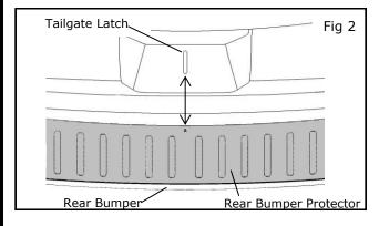
3) Dry fit bumper protector on vehicle by aligning bumper protector centering arrow with tailgate latch.
